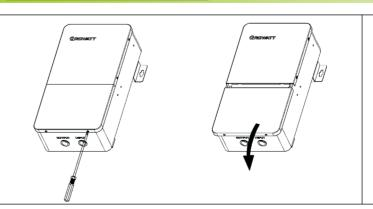
As shown in the picture, please use the screw driver to get out the 2 screws at the bottom of the AT-5000ES, then pull backward to take out the bottom cover.
