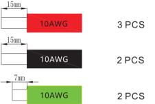
3. There are two types wire need to be machining, please check ref to 9.1 wired diagram. The follow two type wires are show as below (type1 is used to power line connection, type2 is used to ground connection):
