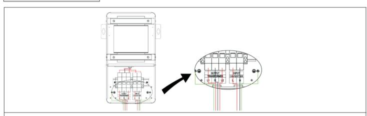
Use the screwdriver to remove the nut on the output terminal strip, and the red 10AWG short wire ends were inserted into the output port L1 and L2, The Black 10AWG short wire ends were inserted into the output port N. Use a screwdriver to lock the ground wire on the earth bus bar.
