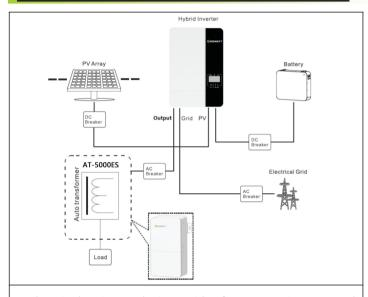
As show in the picture, the input side of AT-5000ES is connected with output of the inverter, and the output side is connected with critical load. There is a transformer in AT-5000ES, it can transform 240V to 120V/240V split phase to provide the power to load.
