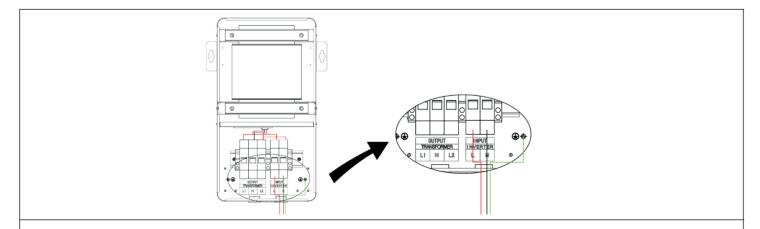
Use the screwdriver to remove the nut on the input terminal strip, and the red 10AWG short wire ends were inserted into the inut port L, the black 10AWG short wire ends were inserted into the input port N. Use a screwdriver to lock the ground wire on the earth bus bar.
